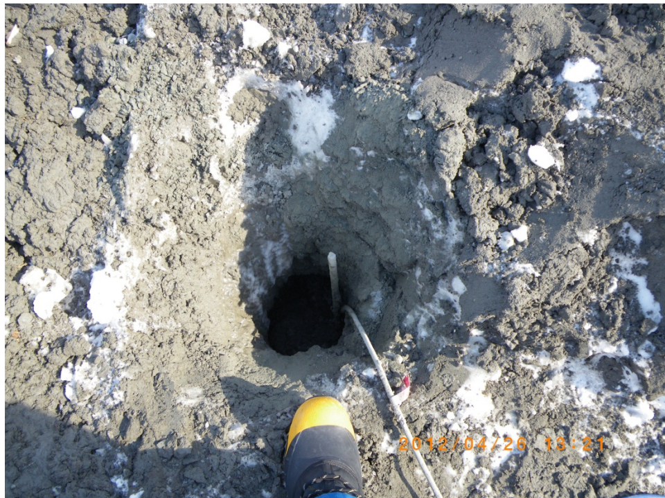
Photo 4: SRK-JT2-12 was secured to a length of rebar.
